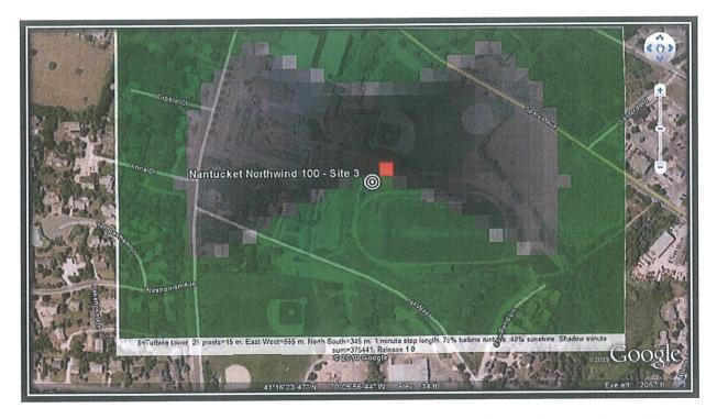
The image above is a shadow plot representing the extent of possible impact from shadow flicker at a distance of 210 meters from the wind turbine. (Fig. 2)
